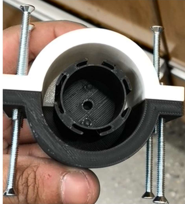
Figure 17. Wheel Mold version two fully assembled prior to filling with silicon
