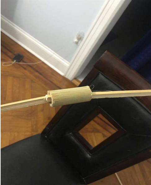
Figure 1: (Collar joint assembled by Khushant)
